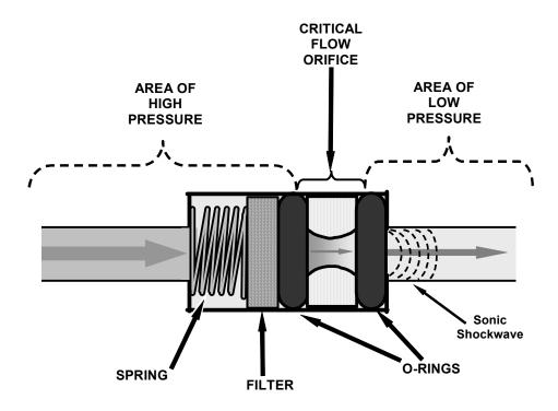
Figure 13-8: Flow Control Assembly & Critical Flow Orifice
